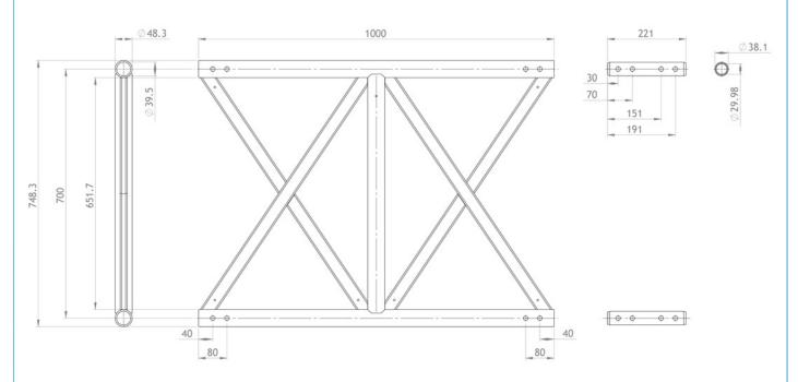
Spigot connections can be introduced at any location in a beam span and don't impact on the beam capacities quoted
