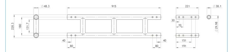
Spigot connections can be introduced at any location in a beam span and don't impact on the beam capacities quoted
