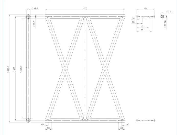
Spigot connections can be introduced at any location in a beam span and don't impact on the beam capacities quoted
